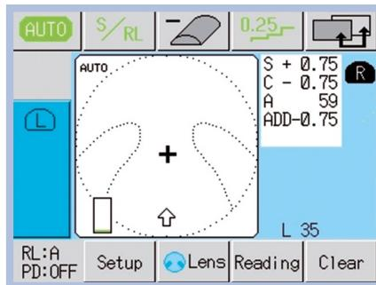
The system detects and measures automatically all progressive lenses. Also modern multi-focal lenses may be measured in FAR, MID and NEAR areas.
