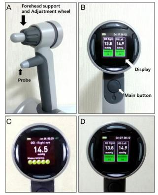
A – forehead support and adjustment wheel; probe. B – display; main button. C – display showing result after measurement on one eye. D – display showing a history of a measurement made on both eyes.
